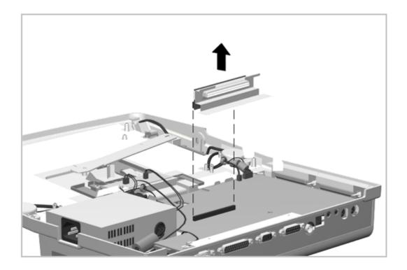
Figure 6-11. Removing the MPEG Connector
